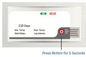
**03** Keep button pressed for minimum 5 seconds to stop recording. Then **ALARM LED** flashed 5 times which indicates a successful stopping.
