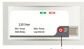
**02** Press button once at any time to check the current status of the logger. See details of these optional features in table below.
