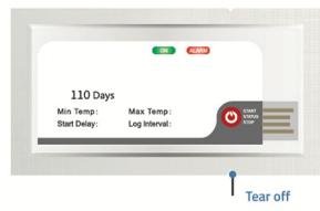
**04** After stopping record, tear off the transparent plastic cover and connect the logger to a USB port of the computer. The PDF and CSV report will be generated automatically and can be found in the device's folder.
