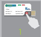
to turn on and enable Innolog™ SU. The data logger is preconfigured and ready to use.
